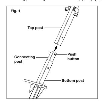
2. Slide the top post over the connecting post until the push button locks into place in its respective hole on the top post (Fig. 2).
